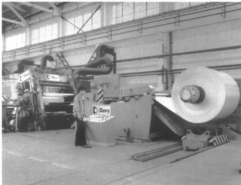
Figure 2.2. Conventional twin-roll caster.
