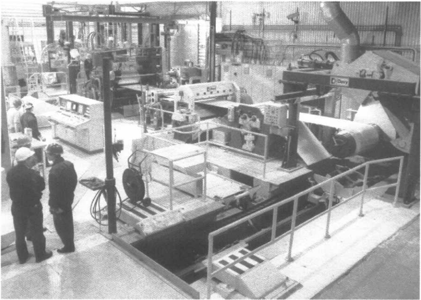
Figure 2.5. The semi-commercial caster installed at Gränges' Finspong facility.
