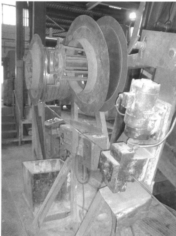
Figure 1.2. System for automatic injection of grain refiner rod into the melt during laundering to the casting machine.
